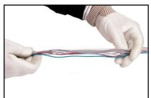
All fiber tubes have got a minimum bend radius. If the tubes are bent below this limit they could break and cause damage the fiber. Splice box made for midspan access sometimes got an oval cable entrance. Apply a radius limiting tool for the tubes when using this type of splice box
