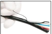
Put the ripcord in the small cut and pull it through the sheath. Keep the ripcord along the cable when opening the sheath.
