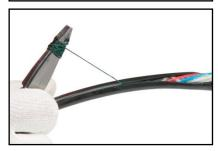
Remove the sheath and cut all the yarns and tapes lying around the fiber tubes. Unwrap the fiber tubes from the reinforcing member (FRP) and cut off the FRP in an appropriate length.
