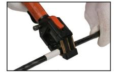
Cut along the cable far enough to expose the cable body and locate the ripcord. Use a tool with controlled cutting depth to prevent damage on the fiber tubes.
