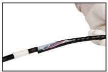
Cut the ripcord and wrap it around the jaws on a plier. Place the ripcord in the small cut and pull it through the sheath. Keep the ripcord along the cable when opening the sheath.
